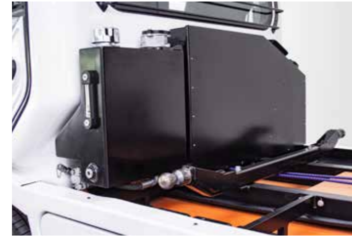
Central hydraulic box compactly integrated behind the cabin, with high power electrical components
