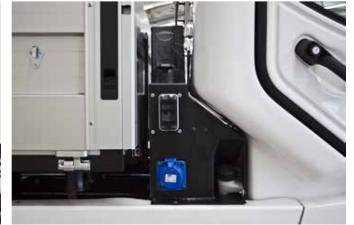
230V / 3000W IP65 connection integrated in the central hydraulic box.
